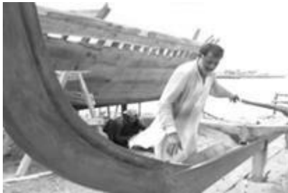
Figure 1: Laying Keel of the Boat with Forefoot and Sternpost. (Source: NCMPR Depository)
